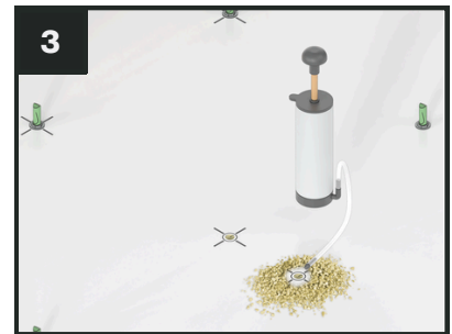
Clean Holes Clean the hole using compressed air to remove all insulation and concrete dust.
